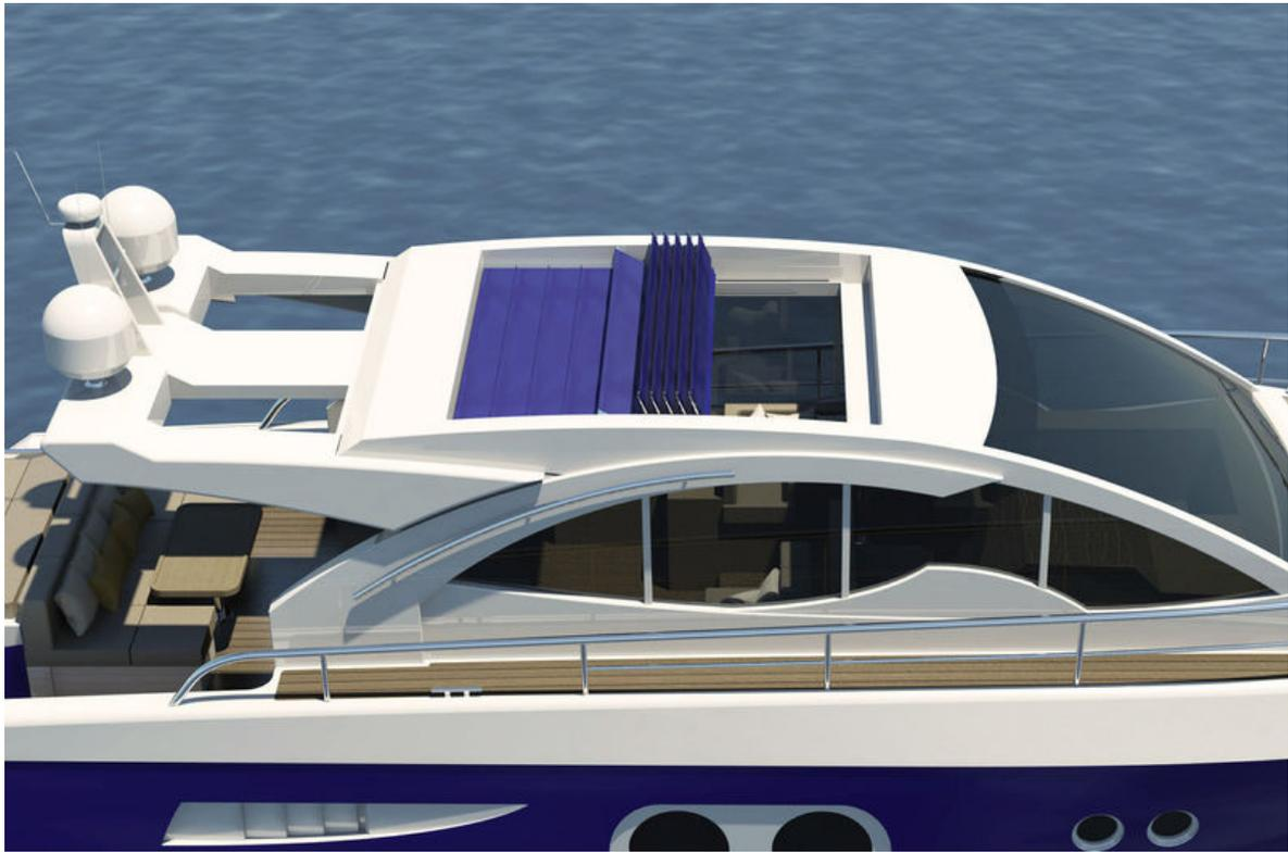
The roof's innovation is simple: it consists in the laminar top itself, which can be opened completely or up to the desired extent. Compared to a similar solution in fabric, the aluminium slats of the top guarantee a longer life and a greater resistance to water and weather.
